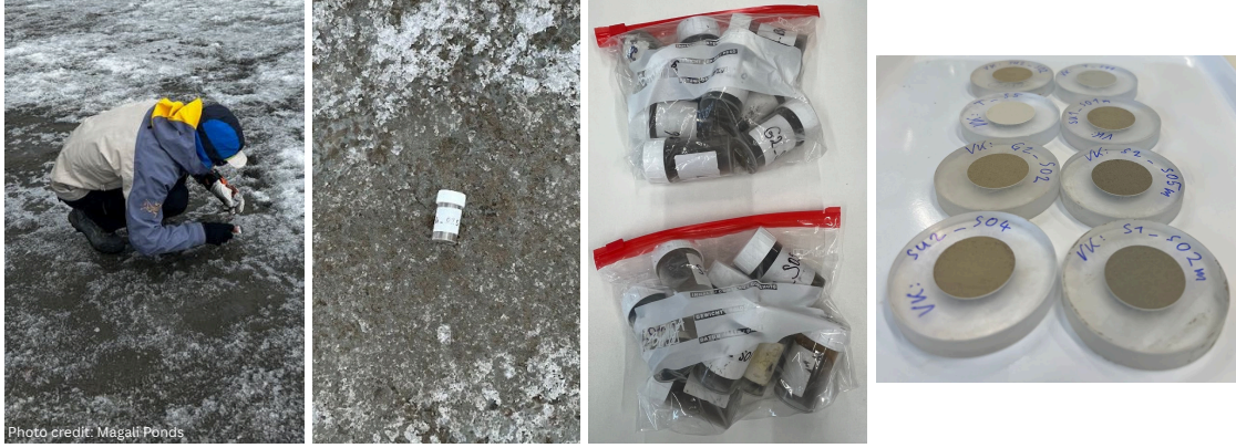
Figure 3: Photos from left to right: Glacier surface deposit sample collection in the field; An exemplary sample tube on top of ice visibly covered with impurities; Sample tube packs arriving in the laboratory; Solid material contained in samples prepared onto disk mounts for XRD analysis.
